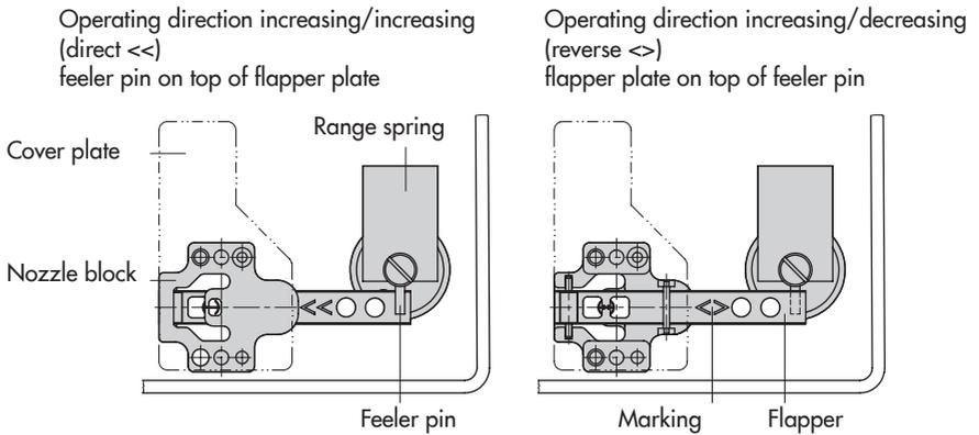
Fig. 9: Position of nozzle block, cover plate removed
