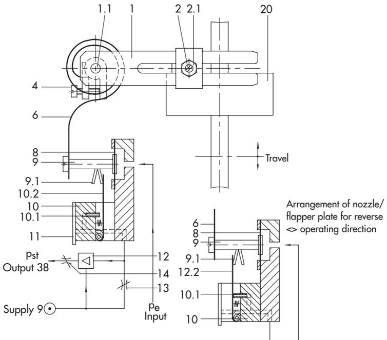
Fig. 2: Functional diagram
