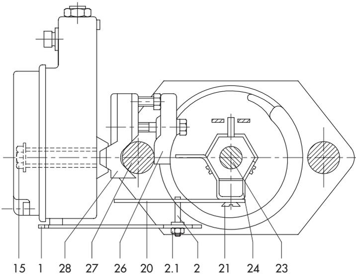
**Fig. 4:** Attachment to valves with rod-type yokes
