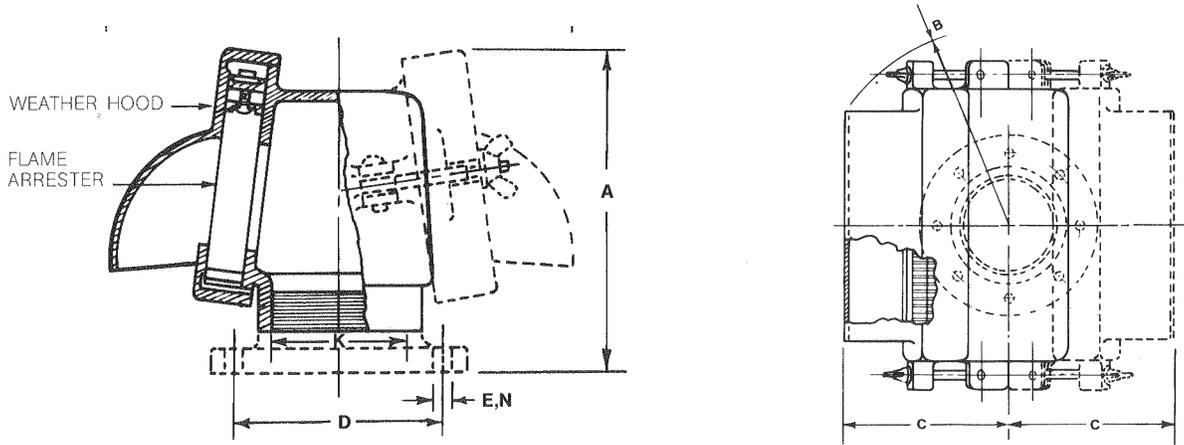
Note: 2" unit has a single flame arresting grid. 3" 4", 6" and 8" units have two flame arrester grids
